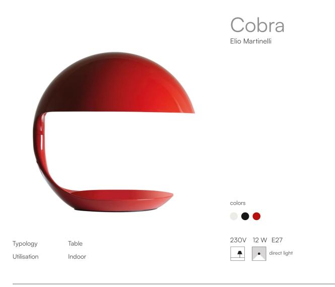
Reading lamp with direct light, made with two resin molded bodies. The lower body part turns on a steel made base connected with the upper body part by means of a central joint for a 360° rotation. The interior reflector is made with white painted aluminium.
