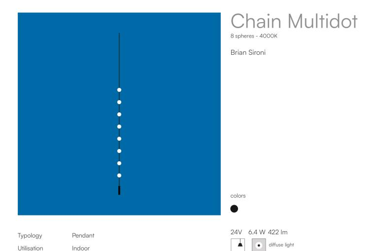
Multidot's cable of 8 spheres has been custom designed to minimise memory and to allow full functionality to be maintained even if a single ball fails. This is made possible by the connections arranged in parallel along the liana: even if one sphere were to be damaged, the system would continue to operate. It is then sufficient to open the damaged sphere and replace the faulty LED, without interrupting general operation. Available colour temperatures are: 2700K, 3000K, 4000K.
